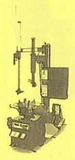
The 70X3 Rim Clamp Tire Changer features Best-In-Class Clamping Capacity (external clamping from 6" to 28" with Grip Max Plus clamp upgrade), Patented Robo-Arm Helper Device to efficiently change low profile or run flat tires, and a Hybrid Duckhead Mount/Demount tool combining advantages of plastic and metal heads.
