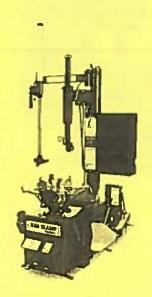
The 70X3 Rim Clamp Tire Changer features Best-In-Class Clamping Capacity (external clamping from 6" to 28" with Grip Max Plus clamp upgrade), Patented Robo-Arm Helper Device to efficiently change low profile or run flat tires, and a Hybrid Duckhead Mount/Demount tool combining advantages of plastic and metal heads.
