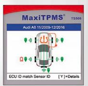
At-a-Glance TPMS Status Screen. Color-coded TPMS Status Screen enables users to diagnose TPMS system at a glance.
