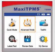
Simplified Interface with Quick and Advanced Modes. Advanced Mode enables users to connect with TPMS system via OBDII port.
