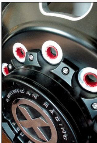
The Counteract Wheel Centering Sleeves in use.
